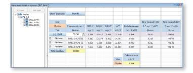
The Supervisor software automatically calculates A(8) vibration exposure value for the time that the contact force was detected. The tools provided with the SV103 enables the user to project the working time with the vibrating equipment as well as removing artifacts from the A(8) calculation. Reports are done in MS Word™ format and can be generated with a single click.
