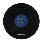
The SV100A measures the A(8) vibration exposure and the overall vibration total value (VECTOR) in accordance with ISO 2631-1 and EU Directive 2002/44/EC. The A(8) result is given in:  $m/s^2$  (RMS),  $m/s^{1.75}$  (VDV) and points. The SV100A monitors the time left to limits and activates the alarm when the limits are reached.
