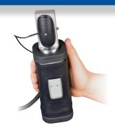
In-situ checks require to use a vibration calibrator such as the SV110 and are intended for checking the instrument's basic calibration and functionality in the field. During the check procedure, the SV107 accelerometer is mounted on the shaker with the SA105A calibration adapter and is excited at vibration level of 10 m/s<sup>2</sup> at 80 Hz. The check procedure lasts 30 s for each axis.
